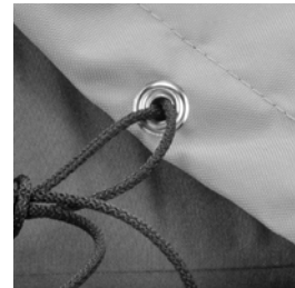
GROMMET Grommets are made of nickel-plated brass and are used primarily on furniture covers to allow a cord to pass through. Grommets can also be used to vent cushions made of vinyl to allow the cushion to breathe.
