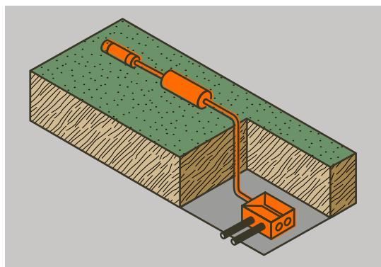
The least conspicuous way to connect an IP44.DE connect system with the mains: the underground connection kit includes a cast resin sleeve to connect the system with the underground cable. The cast resin sleeve is certified to protection rating IP68 and is corrosion-resistant, thus warranting a reliable connection to the power supply that will last for many years.
